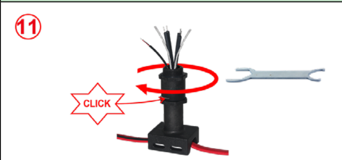
11: Compress the seal by screwing the upper part of the foot. When tightening is complete, a small spring comes to block the assembly (To disassemble, it is necessary to remove this small semi-circular spring). Then it is possible too install this leg through a 32.5mm hole on the selected enclosure.
